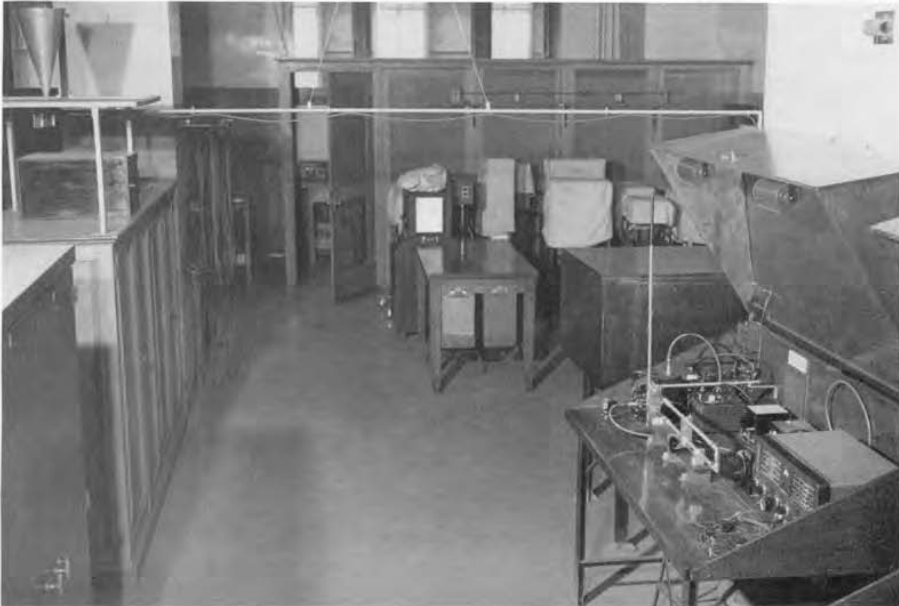
Figure 4. The setup for antenna measurements at very-high and ultra-high frequencies with the Type 1602-A U-H-F Admittance Meter. The cone antenna under measurement is shown at the extreme upper left of the photograph. The special adjustable line can be seen at the front of the test bench.
